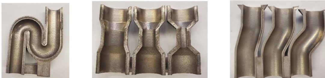
Tubular titanium 6Al-4V AM parts externally & internally smoothed and peened with CASF. Parts are split open in halves for surface roughness and X-Ray diffraction measurements. Photo: Univ. of Washington, Sugino, Joint Center for Aerospace Technology & Innovation.
