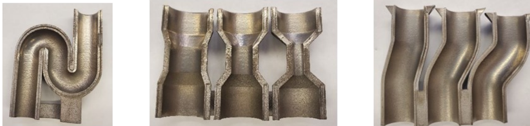
Tubular titanium 6Al-4V AM parts externally & internally smoothed and peened with CASF. Parts are split open in halves for surface roughness and X-Ray diffraction measurements. Photo: Univ. of Washington, Sugino, Joint Center for Aerospace Technology & Innovation.
